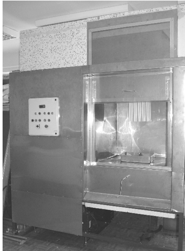
Fig. 5. View of the laboratory impingement stand
