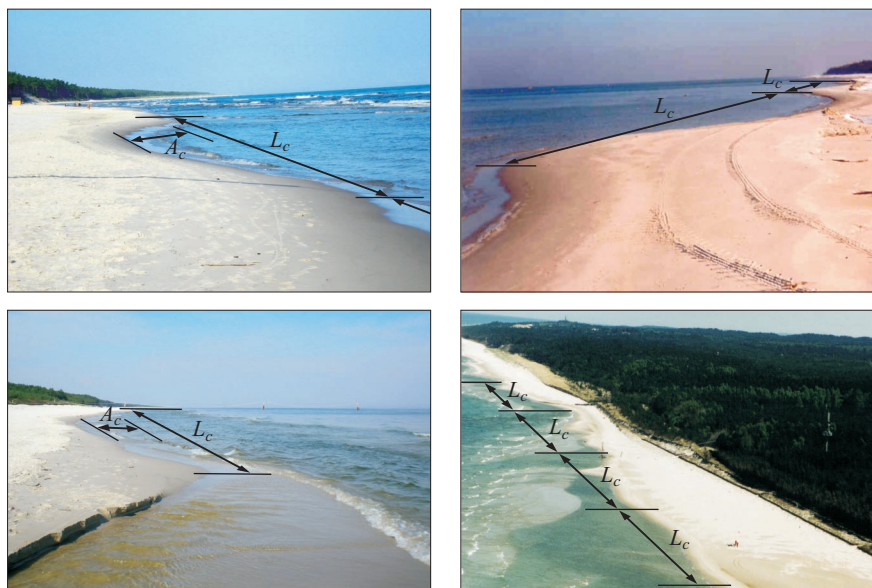
Figure 4. Longshore structure of shoreline rhythmicity patterns ( L_c – cusp wavelength, A_c – cusp indentation length)
