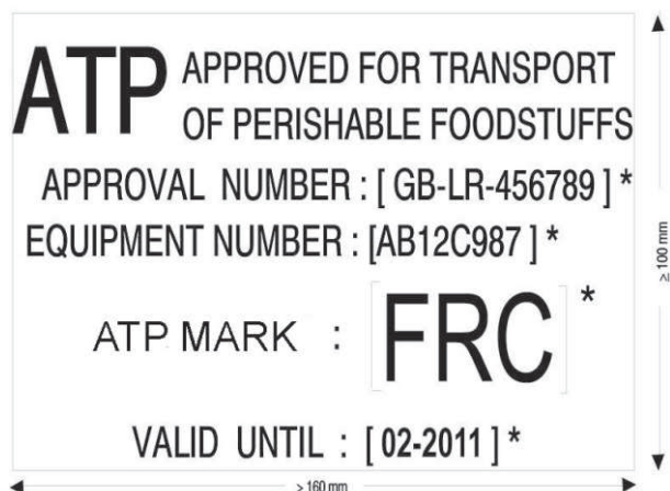
Fig. 1. Certification plate of compliance of the equipment – *the particulars in square brackets are given by way of example [1, 2]
