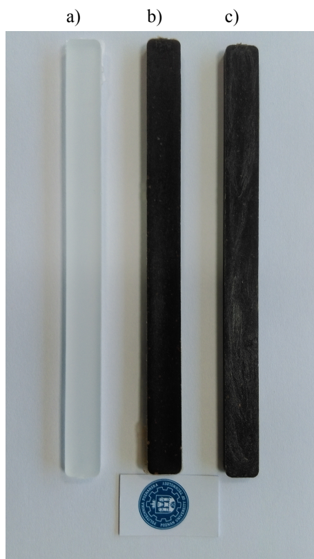
Fig. 2. Selected tensile test specimens of pure PP (a), PP/10NUT (b), PP/10NUT/MAPP (c)
