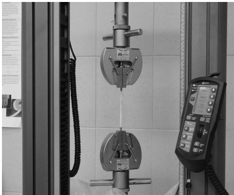
FIGURE 1. Photographs illustrating the types of clamps on an Instron 5966 universal tensile strength testing machine used for measuring the tensile strength of above-ground stems < 16 mm (a) and > 16 mm (b) in diameter
