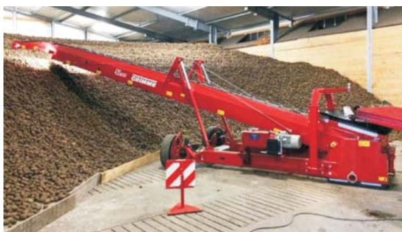
Rys. 6. Pryzmownik do ziemniaków SL 165 [2] Fig. 6. SL 165 potato heaper [2]
