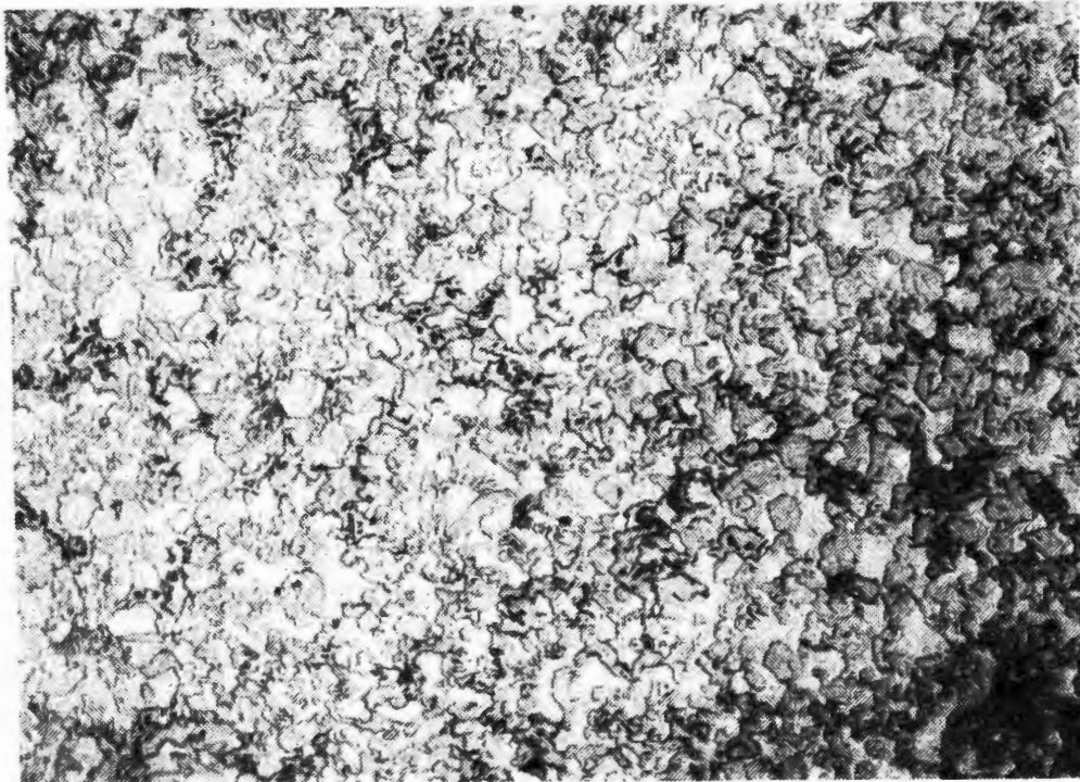
Fig. 7. The microstructure of the material inside the valve head of the stellite homogenizing valve (300x enlargement). Carbides and other intercrystalline phases of spheroidal shape
