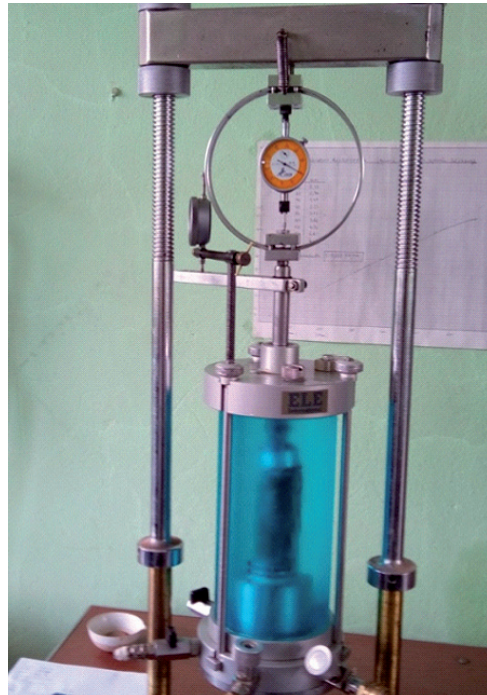
FIGURE 3. The sample of clay prepared for the triaxial test
