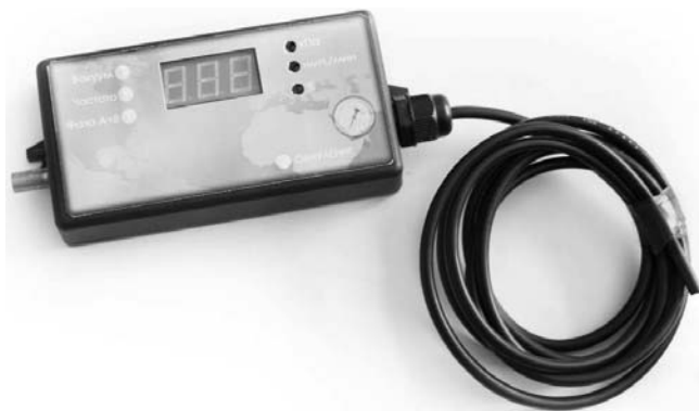
FIGURE 3. The controlling device for the vacuum and pulse parameters of the milking machine
