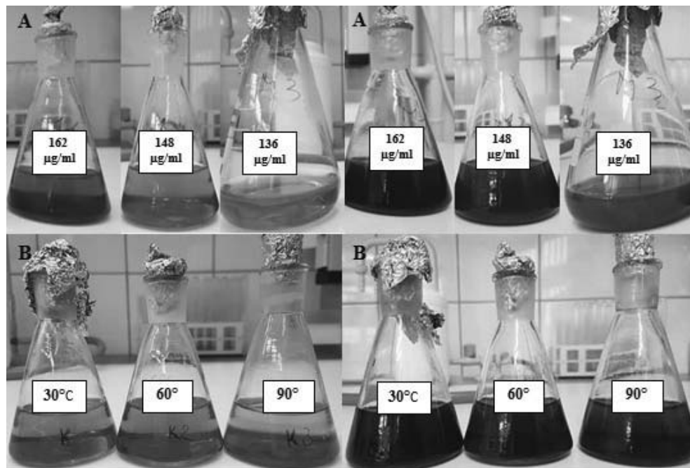
FIGURE 1. Colour change after incubation for 20 and 60 min at room temperature: A – mint-nanosilver, B – cabbage-nanosilver
