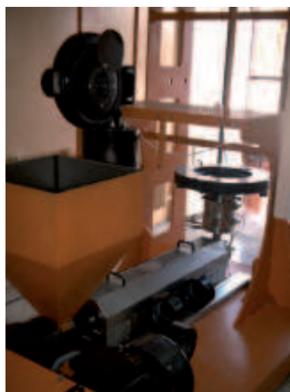
Fig. 1. Stand for film extrusion [14]. The line was produced by SAVO, Wiązowna the Young's modulus and breaking force values determination for the biodegradable film produced from potato starch.
