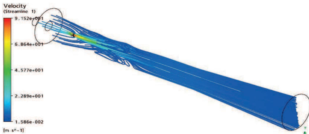
Fig. 4. Lines of Absolute Velocity Fluid Flow in Jet Device of Boiler-Feed Pump.
