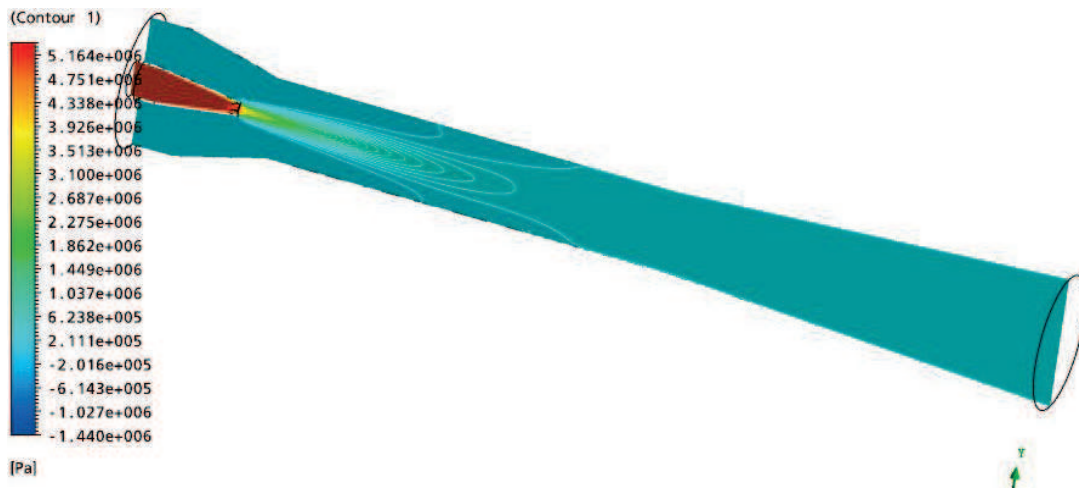
Fig. 6. Hydrostatic Pressure Distribution Pattern in Jet Device of Boiler-Feed Pump.
