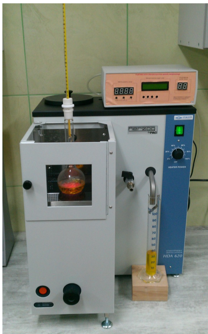
Fig. 2. Photo bench equipped with a distiller HAD 620/1 by Herzog
