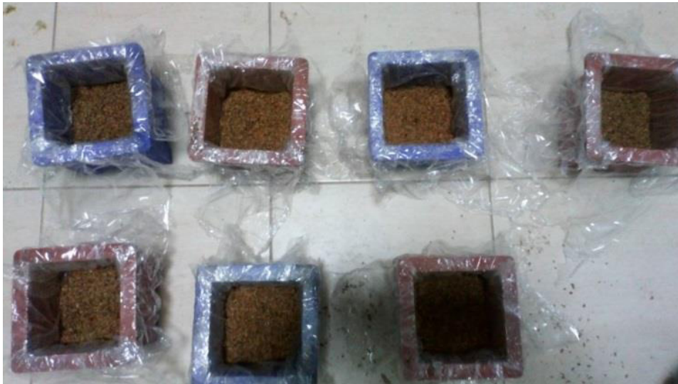
Fig. 3. Production of insulation board samples
