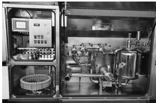
Figure 11. Cabinet interior with installation for milk collection and analysis at the tanker
