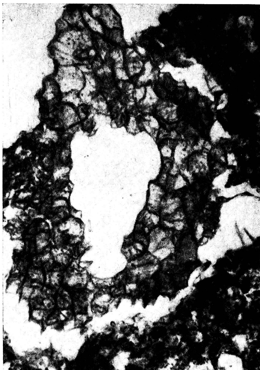
Fig. 4. Small-grained calcite in a pore-chamber of typical thick chernozem, Kursk region ( \times 150 ).
