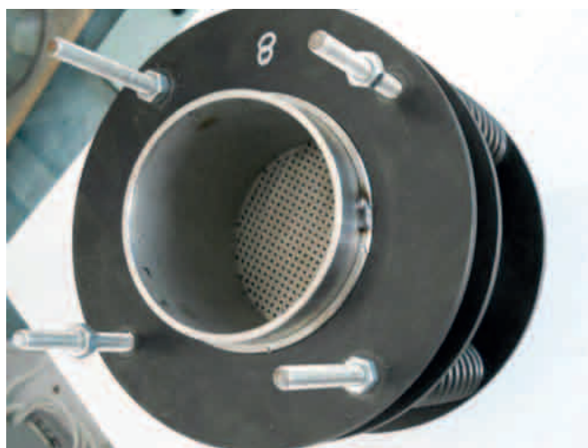
Fig. 1. Specially designed silo-stress simulator vessel
