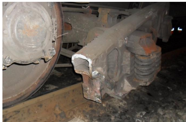
Fig. 1. Typical breakdown of bogie side frames
