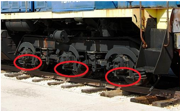
Fig. 2. Axle-box lines (locomotive TEM3)
