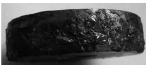
Fig. 9. Erosive wear of roller at affecting of electric current of high-density tribounit of "roller-rail" at presence of sand
