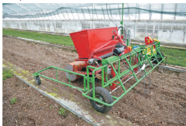
Fig. 2. A functional model of the unit suspended asymmetrically on the arm of the tractor precision seeder, designed for work in nursery seedbeds
