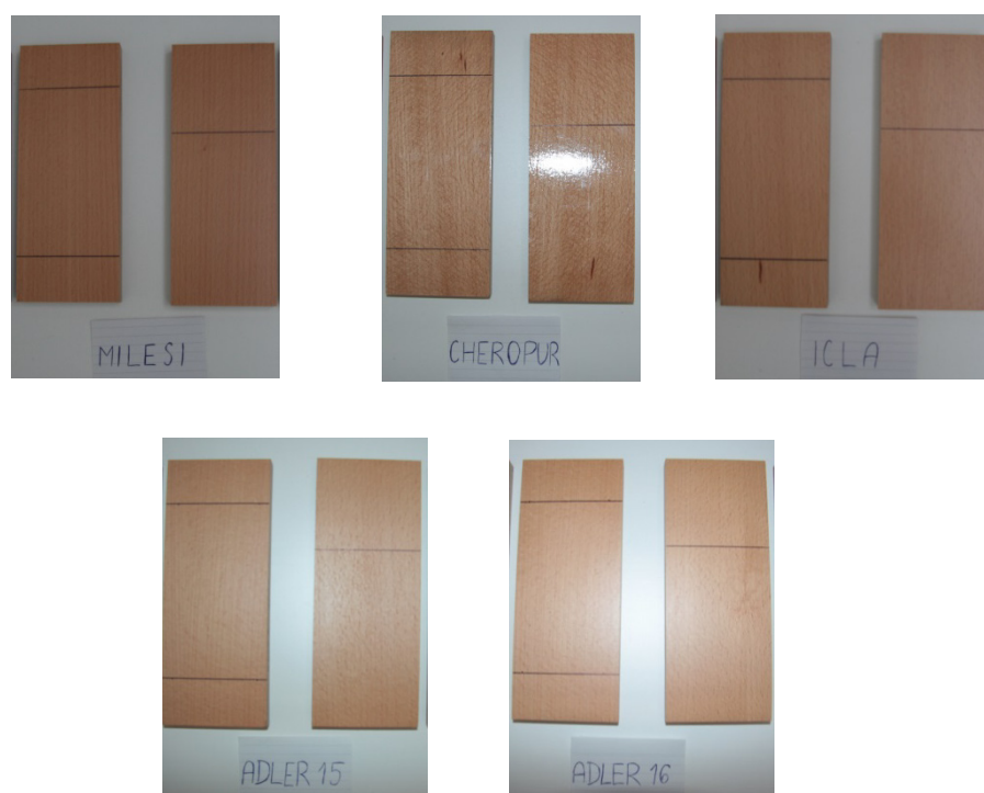
Fig. 1 The test specimens according to STN EN 11925-2 – before the test of ignitability
