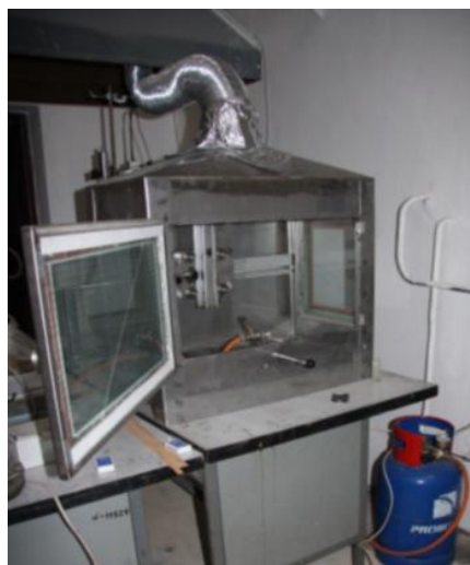
Fig. 2 The test device equipment according to STN EN 11925-2
