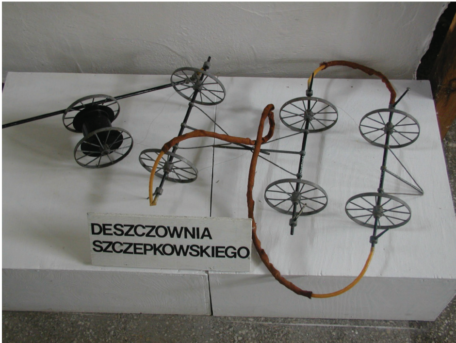
Photo 1. Szczepkowski's sprinkler irrigation machine model at the National Museum of Agriculture and Agri-Food Industry at Szreniawa (photo by Roman Rolbiecki)
