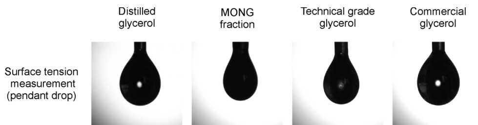
Fig. 2. The recorded images of the surface tension measurements, using the pendant drop method, of the tested biofuel by-products (distilled glycerol, technical grade glycerol, the MONG fraction) and commercial glycerol.
