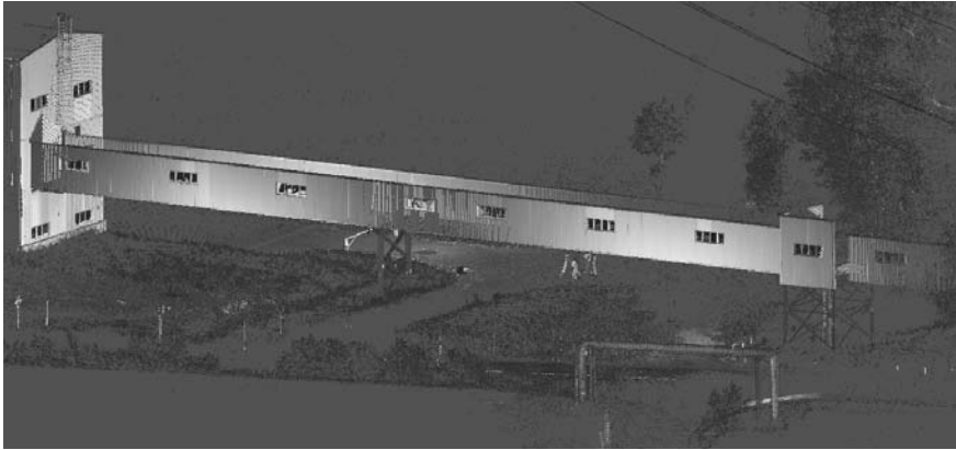
FIGURE 3. Fragment of a global point cloud after absolute orientation
