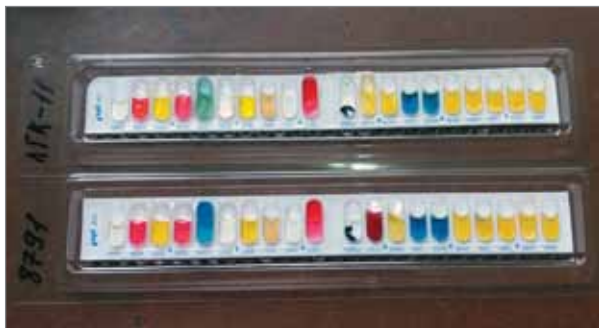
Figure 8. Characteristics of isolate 11 using API 20E test system
