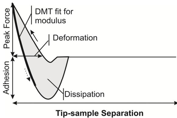
Fig. 1 Tip force vs. tip-sample separation
