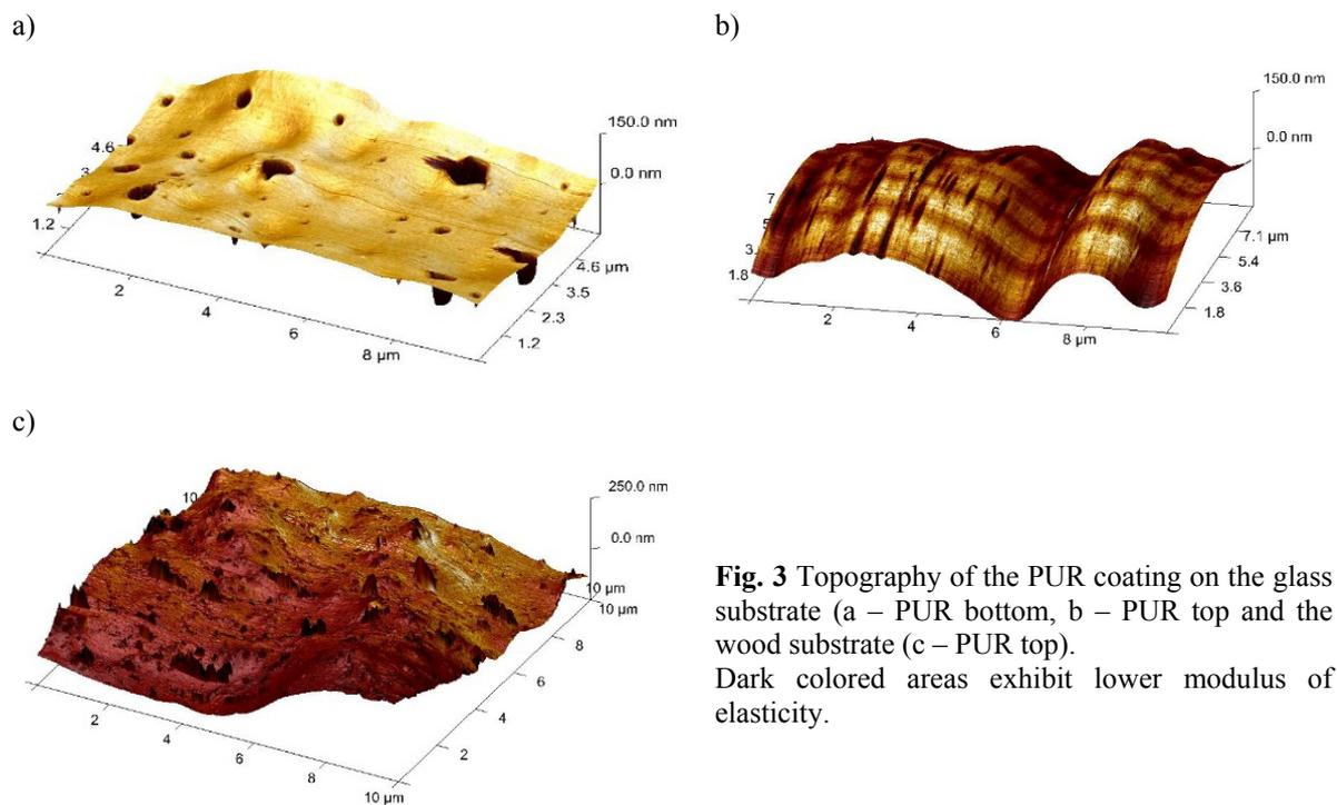
**Fig. 3** Topography of the PUR coating on the glass substrate (a – PUR bottom, b – PUR top and the wood substrate (c – PUR top). Dark colored areas exhibit lower modulus of elasticity.
