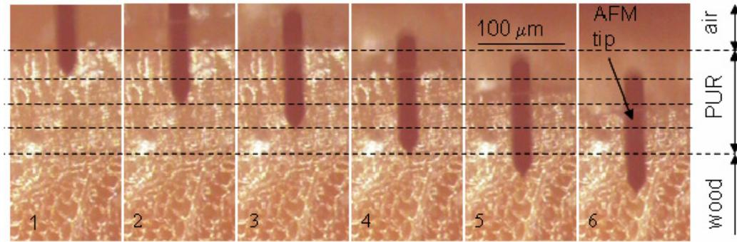
**Fig. 2** Positions of the measuring AFM tip at the wood – PUR coating interface. The position 1 is within the 4<sup>th</sup> layer of the coating, position 4 is within the 1<sup>st</sup> layer of the coating, and positions 5 and 6 are the positions within the wood cell wall.
