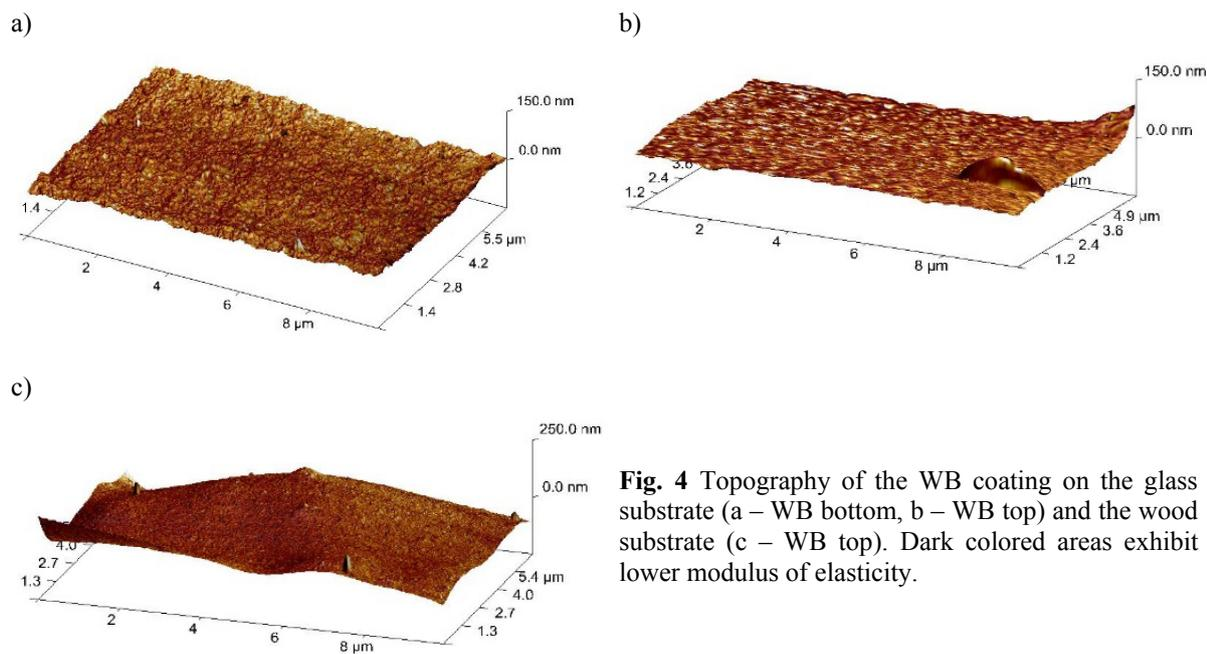
**Fig. 4** Topography of the WB coating on the glass substrate (a – WB bottom, b – WB top) and the wood substrate (c – WB top). Dark colored areas exhibit lower modulus of elasticity.
