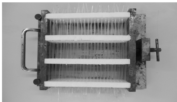
Fig. 6. Modified forms to make the translucent concrete specimens
