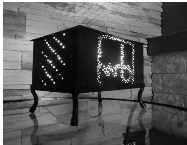
Fig. 11. decorative element in form of the lamp made of the translucent concrete
