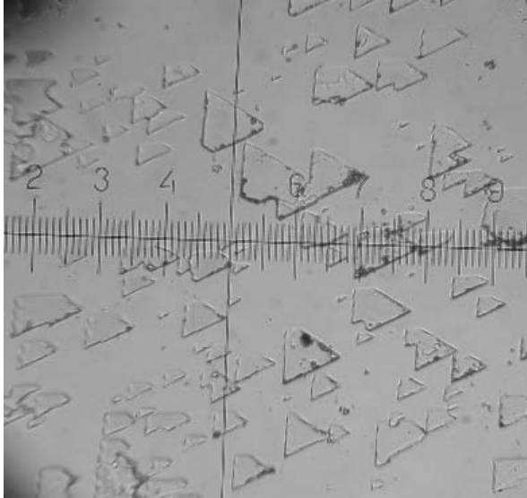
Fig. 2. The morphology of surface of ES grown on gallium arsenide substrates with orientation (111)
