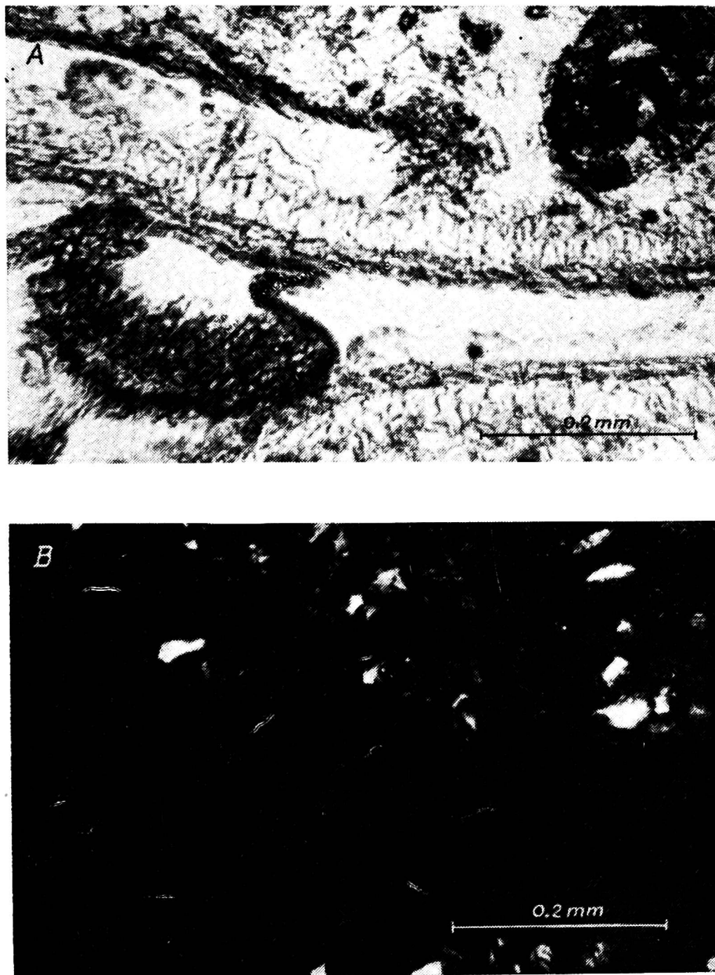
Fig. 1. Micromorphology of brown soil developed from loess. Horizon A_1 , sampling depth 3-13 cm. Fragments of plant remains in initial humifying state. A — in plain light, B — under crossed polarizers.
