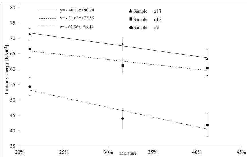
Legend: Unitary energy [ $\text{kJ}/\text{m}^2$ ], ▲ – stem diameter 13 [mm], ■ – stem diameter 12 [mm], ● – stem diameter 9 [mm], Moisture [%],
