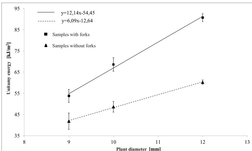
Legend: Unitary energy [kJ/m<sup>2</sup>], ■ – stem with forks, ▲ – stem without forks, Stem diameter [mm]
