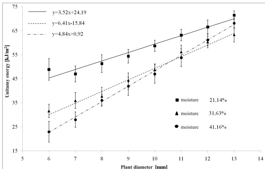
Legend: Unitary energy [kJ/m<sup>2</sup>], ■ – moisture 21,14%, ▲ – moisture 31,63%, ● – moisture 41,16%, Stem diameter [mm]
