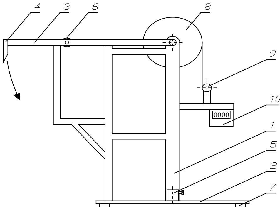
Fig. 3. Measuring device of pendulous type: 1 – mast with frame, 2 – main plate, 3 – pendulum, 4 - knife, 5 – holder of plant sample with fastening handwheel, 6 – stop dog, 7 – adjustable foot, 8 –rotary disk, 9 – linear transducer, 10 – digital recording device.
