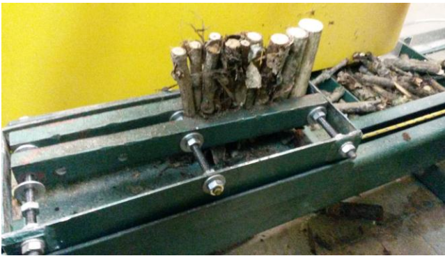
Fig. 3. Truck with the poplar's samples placed on the guide rail
