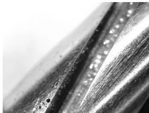
Fig. 5. A seized component of the plunger and barrel assembly of a fuel injector's needle
