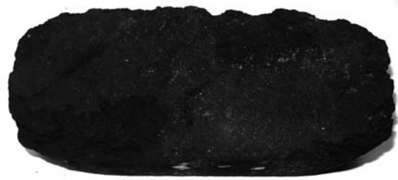
Fig. 3. Briquette from oak pulp
