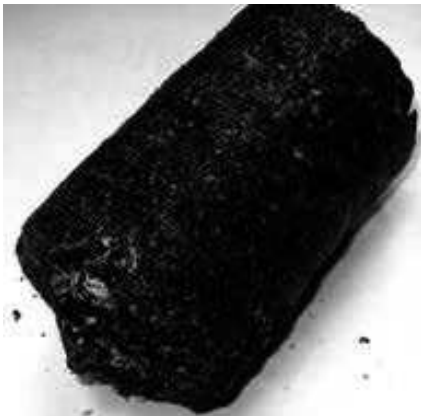
Fig. 6. Briquette from sunflower shells
