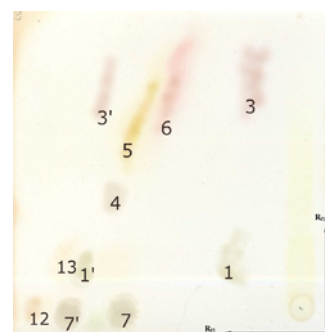
Fig. 2 2D TLC chromatogram of fractions F b of phenolic acids from the flowering herb Cirsium vulgare (Savi) Ten. Direction I: benzene-methanol-acetic acid-acetonitrile (80:10:5:5) v/v. Direction II: sodium formate-formic acid-water (10:1:200) w/v/v. The spots were visualized with diazotized sulfanilic acids (dSa) in 20% sodium carbonate solution 1:1 v/v. 1,1' – caffeic acid; 3,3' – synapic acid; 4 – gentisic acid; 5 – vanillic acid; 6 – syringic acid; 7 – chlorogenic acid; 12 – unknown compounds; 13 – unknown compounds.
