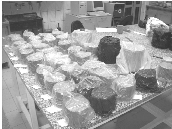
FIGURE 2. Samples after the Proctor test and CBR molds
