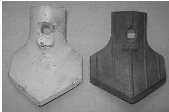
Fig. 8. Duckfoot share for spring cultivator teeth made by forging and welding (left) and as a casting (right (own construction))
