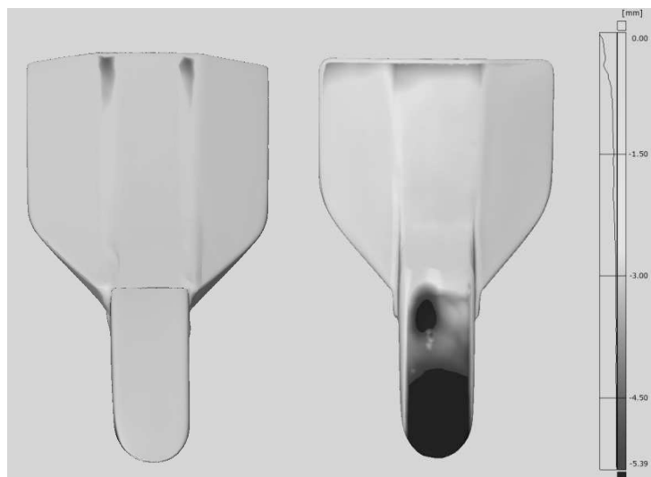
Rys. 7. Comparison of subsoiler plough wear intensity, welded construction (left) and casting (right) [own research]
