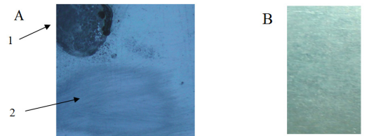
Fig. 3. A – surface of cleaving saw with applied zinc coating: 1 – the effect of nitric acid, 2 – the effect of sanding; B – section of cleaving saw prepared for coating thickness testing
