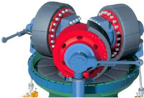
Fig. 3. General view of the grinding table and rollers with the replaceable segments
