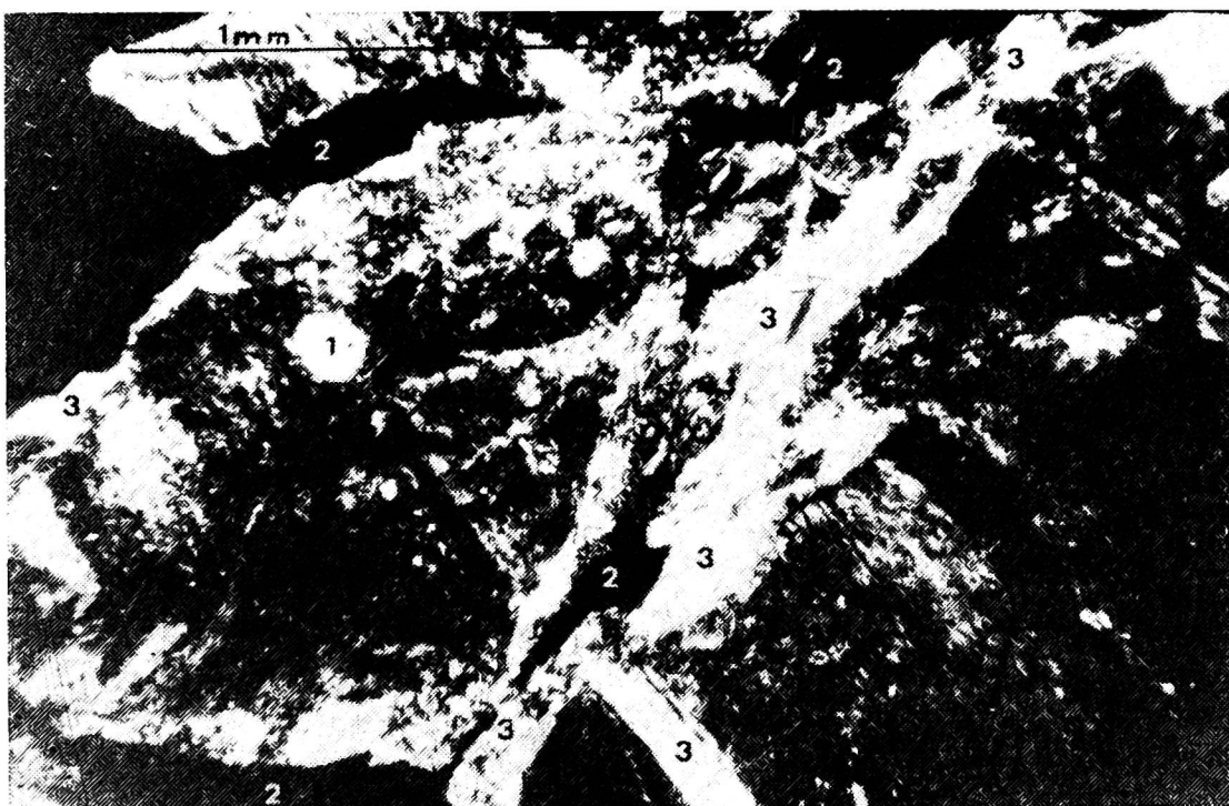
Fig. 2. B 3tg of a "lessivé" soil developed on clayey continental sediments of the Chateauroux forest (crossed nicols). The fragments of clayey sediment are coated with thick, yellowish white argillans with strong continuous birefringence. 1 — quartz, 2 — void, 3 — free grain argillan.
