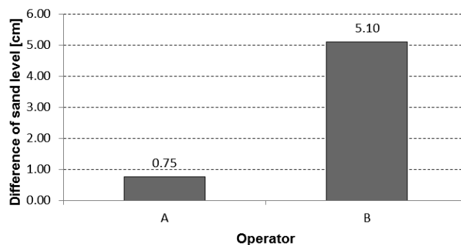
FIGURE 5. Comparison of sand level differences (before and after sand spreading) for two evaluated operators: “A” and “B”
