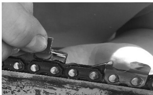
FIGURE 2. The method of taking the cutting edge imprint
