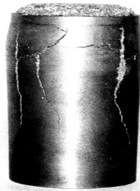
Fig. 2. Destruction of the chamber during densification ( p_k – approx. 145 MPa)
