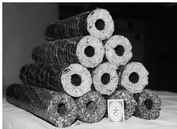
Fig. 6. Briquettes (from spruce sawdust, from spruce sawdust with a buckwheat hulls content) [2]
