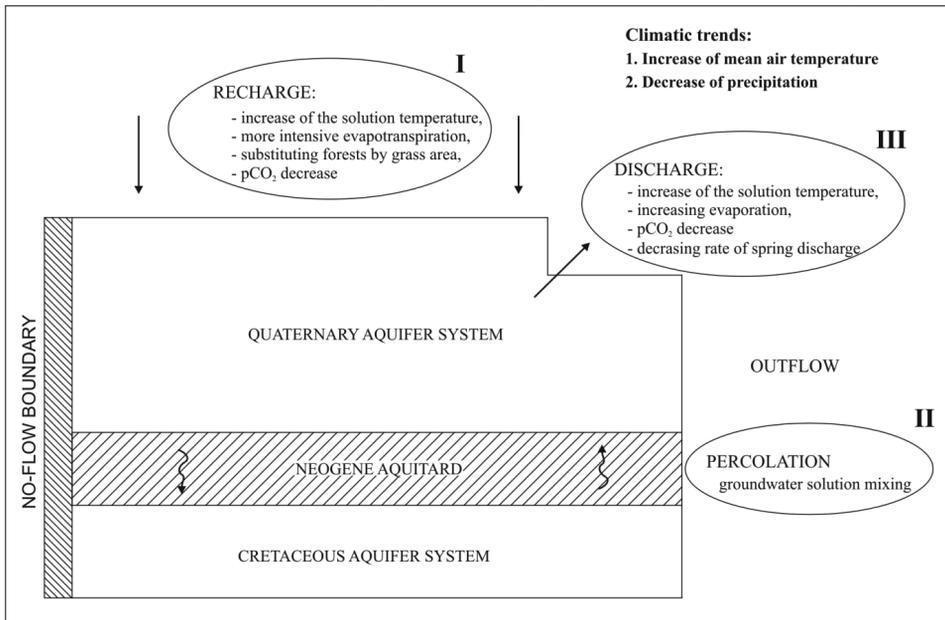
Fig. 6. Schematic model of the multi-aquifer system in the cupola area
