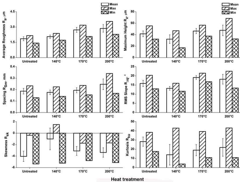
**Fig. 4.** L Roughness parameters obtained for measurements perpendicular to wood grain at the different heat treatments
