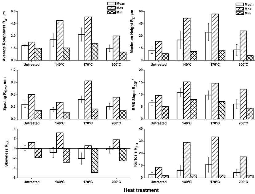
**Fig. 3.** Roughness parameters obtained for measurements parallel to wood grain at the different heat treatments
