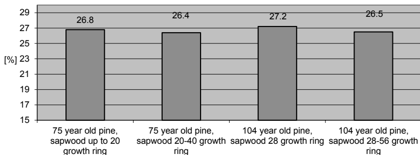
Fig. 5. The content of lignin in pine sapwood with division into growth ring zones
