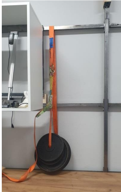
Fig. 9. Empirical testing of frame stiffness and element deflections using weights in a situation simulating the suspension of the cabinet lifting and lowering system.
