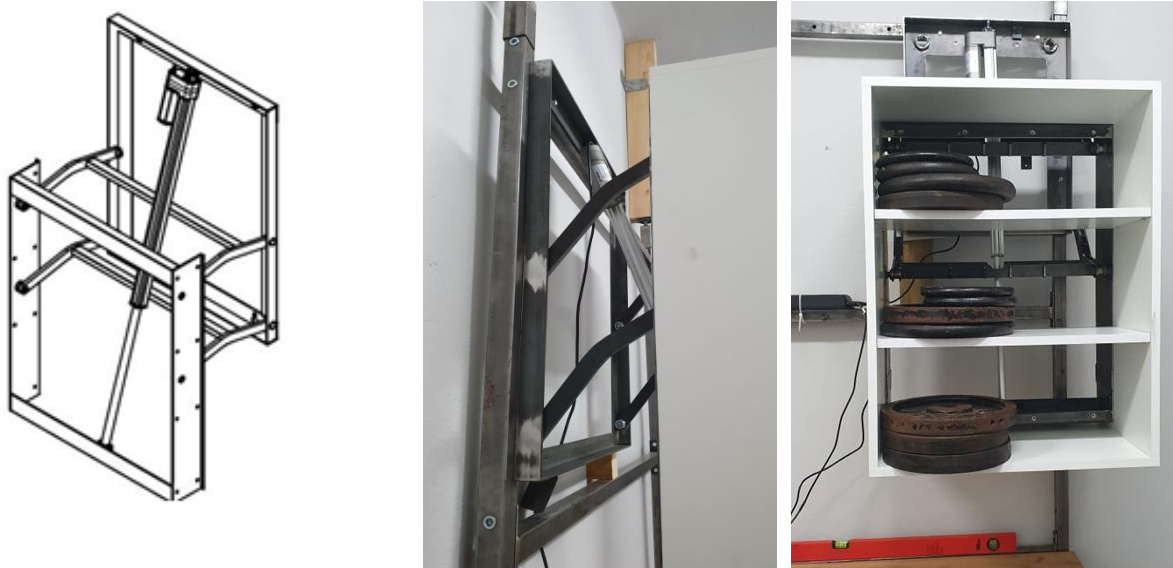
Fig. 10. Schematic diagram of the upper cabinet mechanism, side view of the prototype mechanism with the cabinet, cabinet with the mechanism during tests with asymmetric loading.
