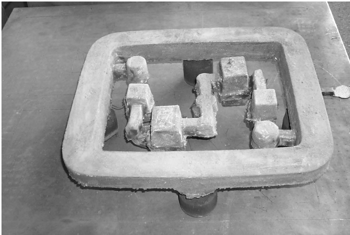
Fig. 2. View of the lower part of casting with a set of chambers for spheroidisation and inoculation
