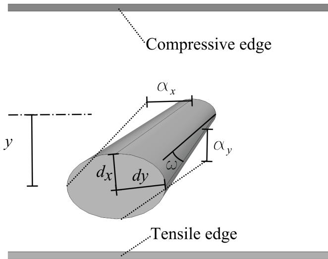
**Fig. 2. Geometry of the knots in the model, including the measuring parameters: position ( $y$ ), minor ( $d_x$ ) and major ( $d_y$ ) semi-axis, conical angle ( $\omega$ ), and vertical ( $\alpha_y$ ) and horizontal ( $\alpha_x$ ) inclinations**
