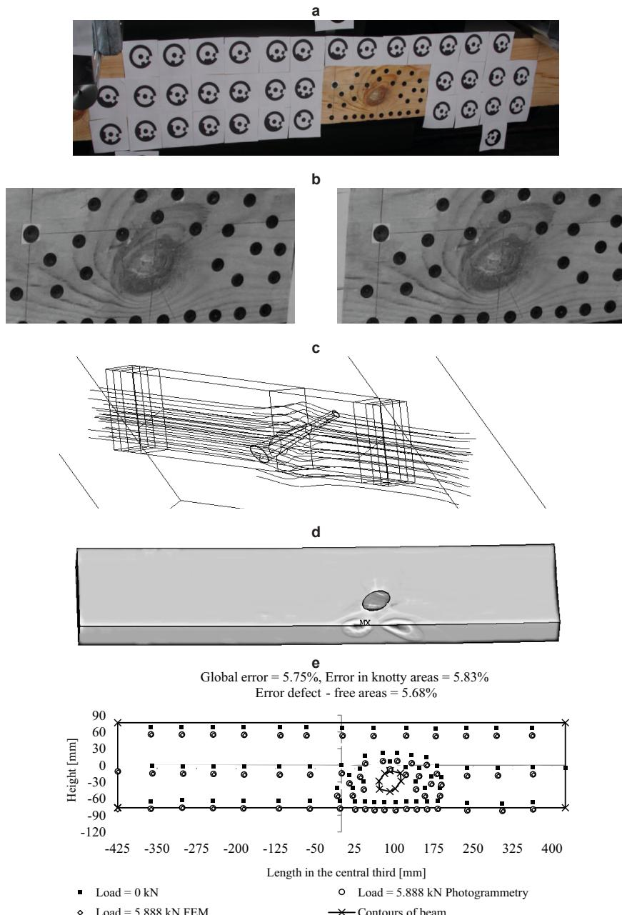
**Fig. 4. Experimental and numerical validation.** (a) Photogrammetric measuring points in each beam. (b) Detection of knot, location and load of failure via image correlation. (c) Numerical simulation of knot of failure and grain deviation. (d) Calculation of failure criteria (Hoffmann criterion shown in the image). (e) Comparison of photogrammetric versus numerical displacements
