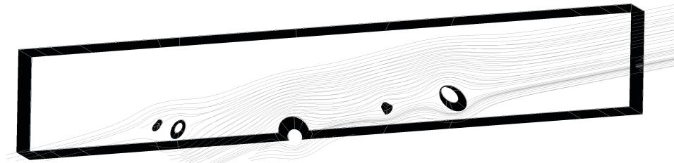
**Fig. 3. Fiberorientation according to flow-grain analogy.** The figure shows the load span (see fig. 1.) of a beam including the knots and the fiber orientation. The fiber orientation is accounted for in the model by simulating a laminar flow around the knots and reorienting the orthotropic directions
