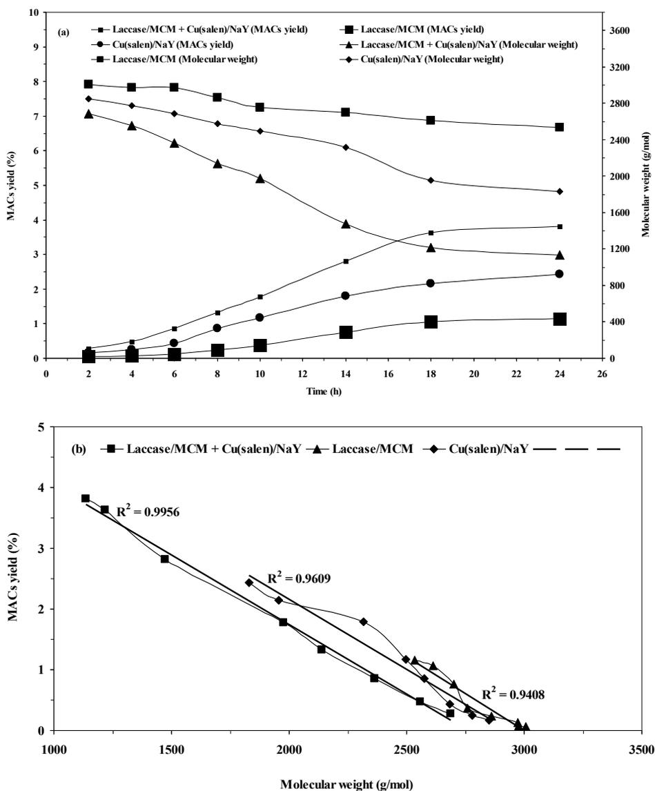
**Fig. 2.** MACs yield and Mw of kraft lignin: a – effect of reaction time, b – relation between MACs yield and molecular weight of kraft lignin. Reaction temperature: 80°C; laccase/MCM-to-Cu(salen)/NaY ratio 1:1 (wt %)
