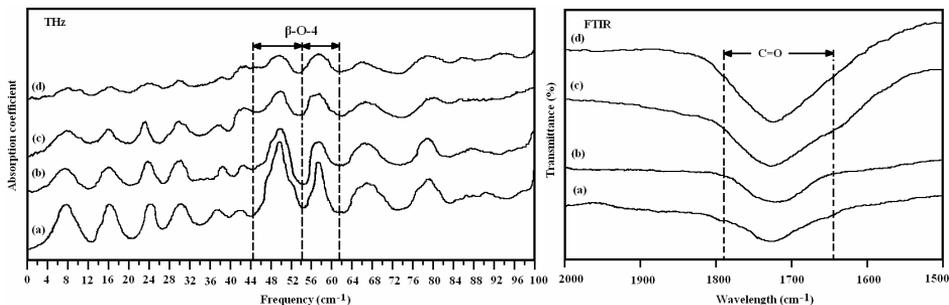
**Fig. 3.**  $\beta$ -O-4 linkage (THz spectra) and carbonyl group (FTIR) in kraft lignin: a – kraft lignin, b – kraft lignin after treatment with laccase/MCM, c – kraft lignin after treatment with Cu(salen)/NaY, d – kraft lignin after treatment with laccase/MCM + Cu(salen)/NaY. Reaction temperature: 80°C; reaction time: 18 h; laccase/MCM-to-Cu(salen)/NaY ratio 1:1 (wt %)
