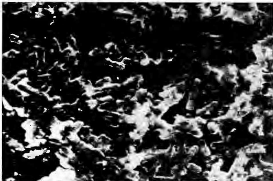
Fig. 3. B. subtilis on polished aluminium before cleaning. Carrier — 0.85% NaCl, magnification 3000 \times
